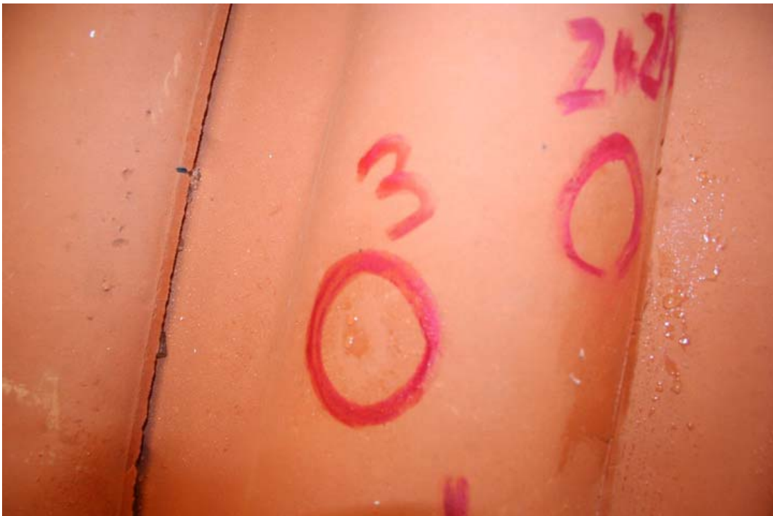
A-12. Tile 1 at impact 3 with 1-1/2 inch ice ball.
