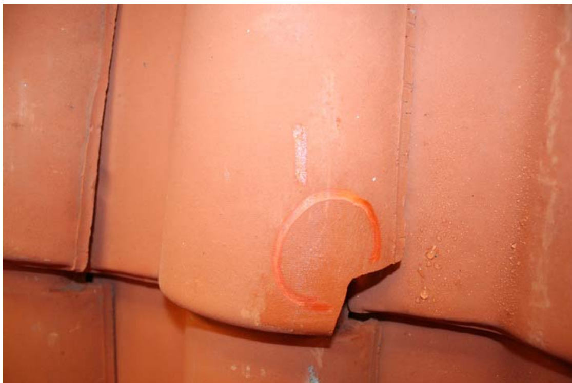
A-52. Tile 5 at impact 1 with 1-3/4 inch ice ball; note fracture.
