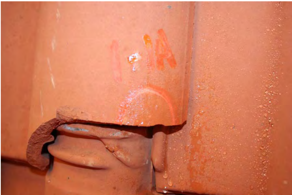
A-48. Tile 4 at impact 1A with 1-3/4 inch ice ball; note fracture.
