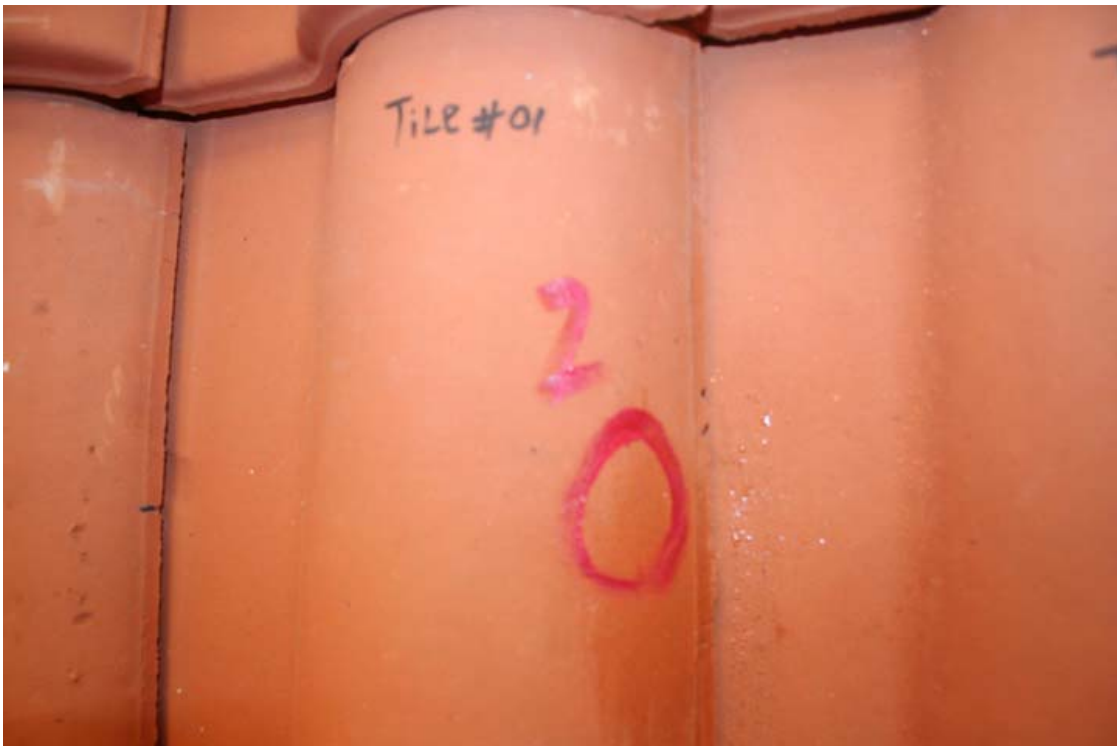
A-8. Tile 1 at impact 2 with 1-1/2 inch ice ball.
