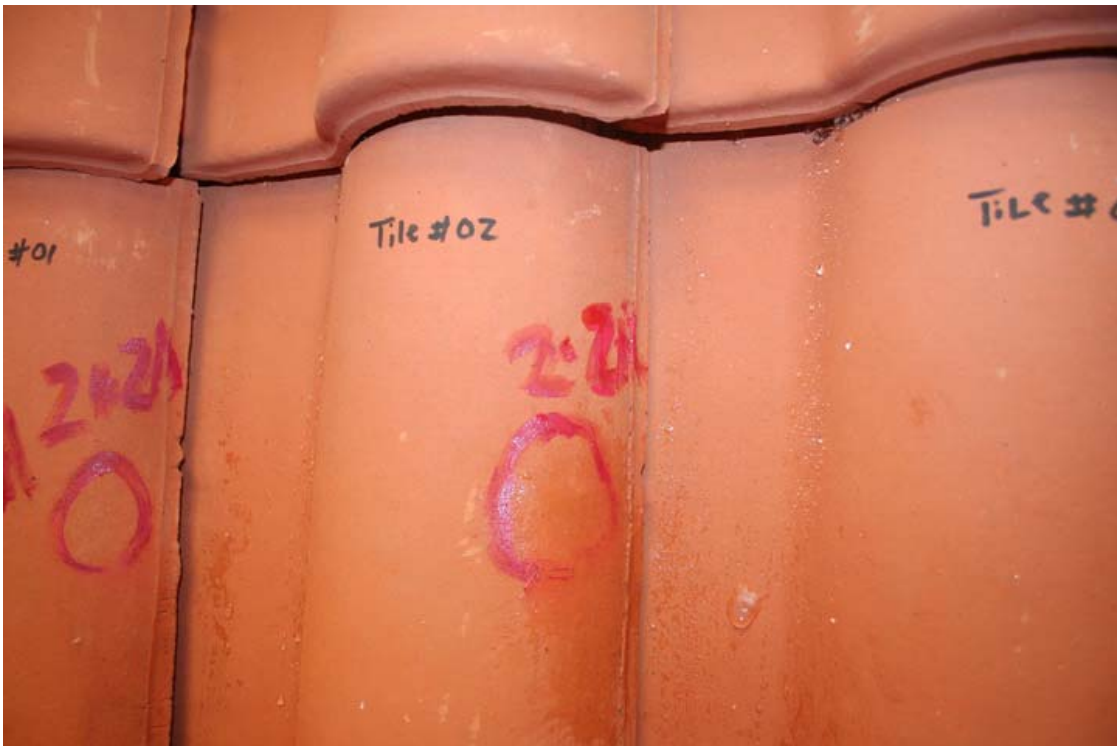
A-24. Tile 2 at impact 2A with 1-1/2 inch ice ball.
