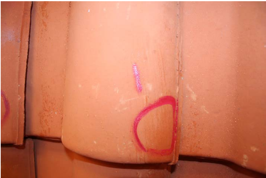
A-18. Tile 2 at impact 1 with 1-1/2 inch ice ball.
