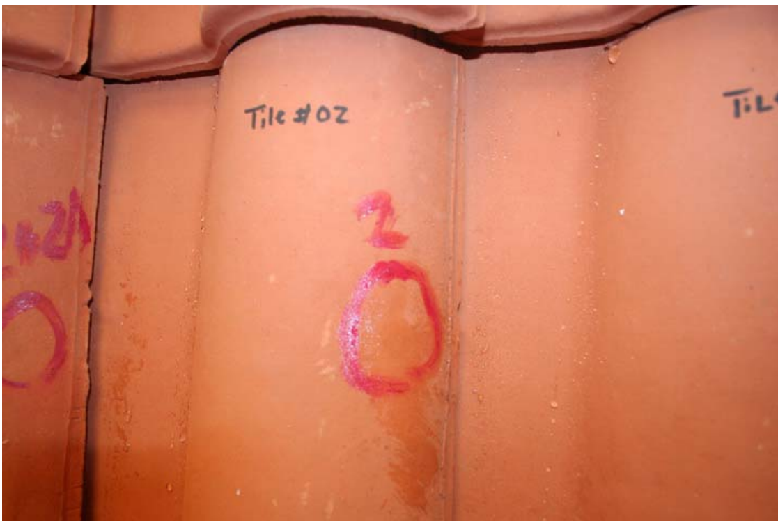
A-22. Tile 2 at impact 2 with 1-1/2 inch ice ball.
