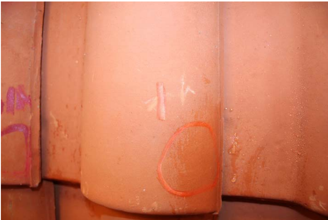
A-32. Tile 3 at impact 1 with 1-3/4 inch ice ball.
