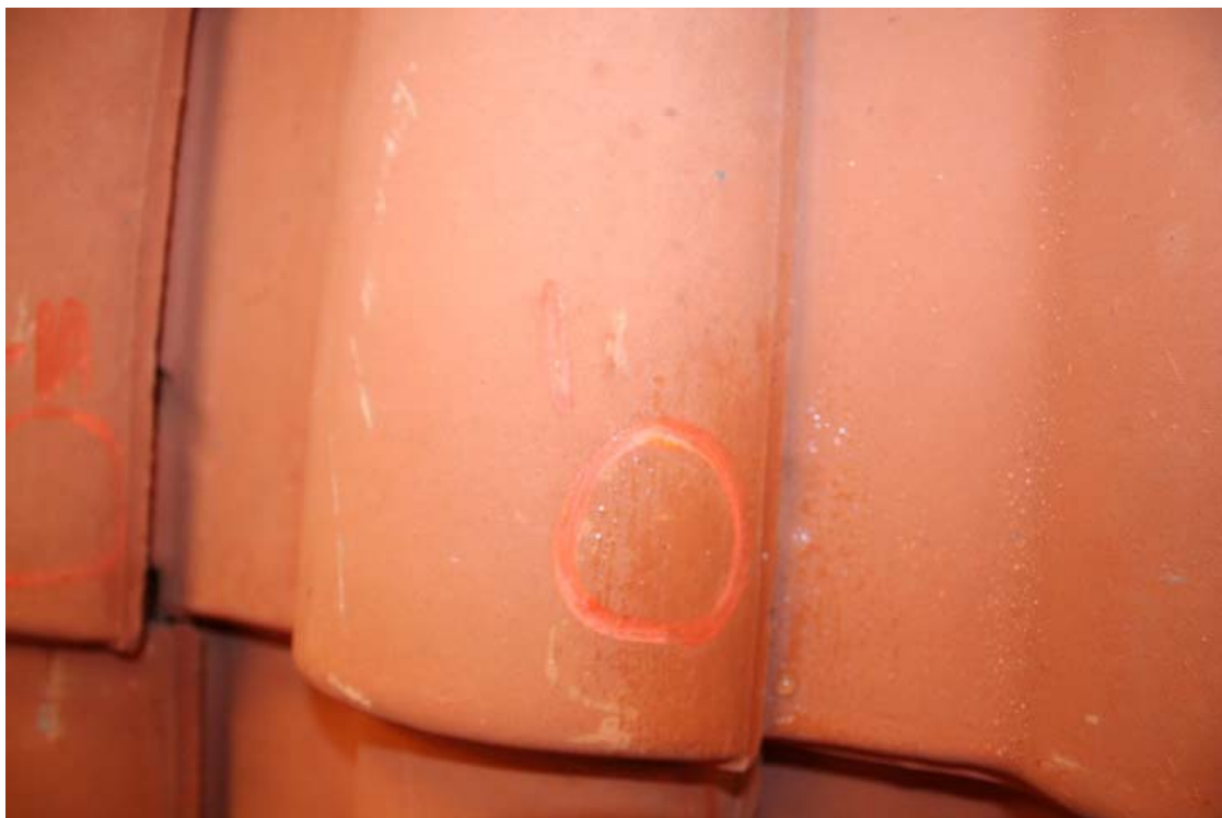
A-46. Tile 4 at impact 1 with 1-3/4 inch ice ball.
