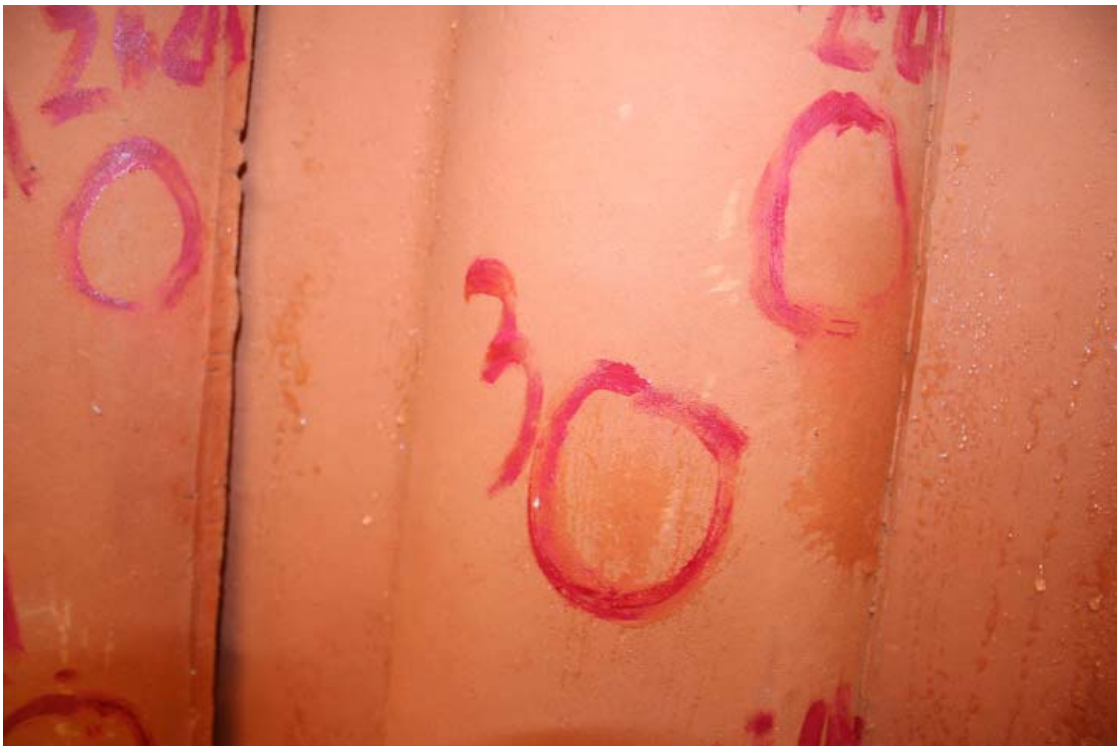
A-26. Tile 2 at impact 3 with 1-1/2 inch ice ball.
