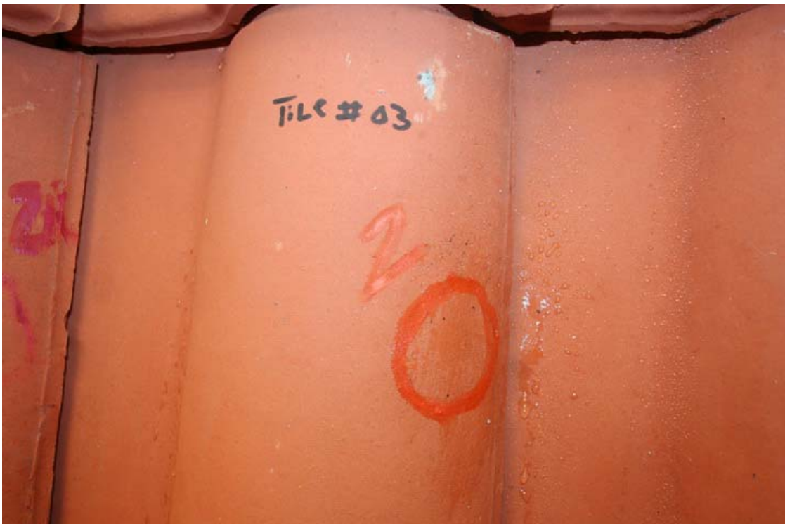
A-36. Tile 3 at impact 2 with 1-3/4 inch ice ball.
