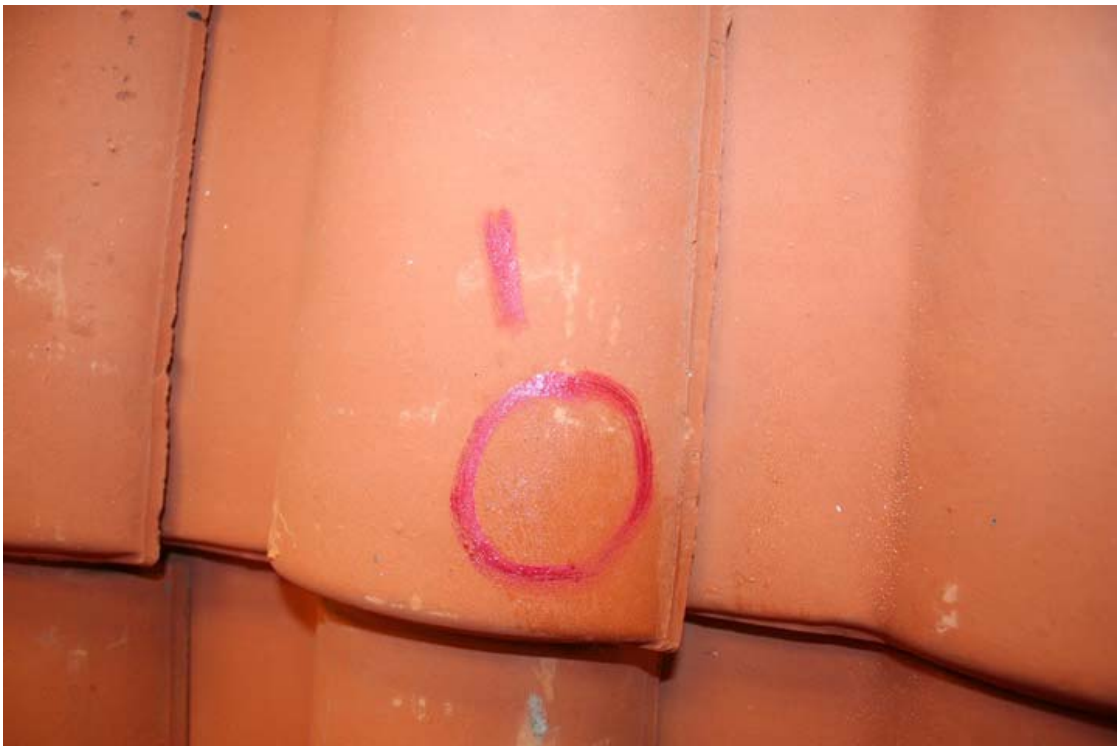
A-4. Tile 1 at impact 1 with 1-1/2 inch ice ball.
