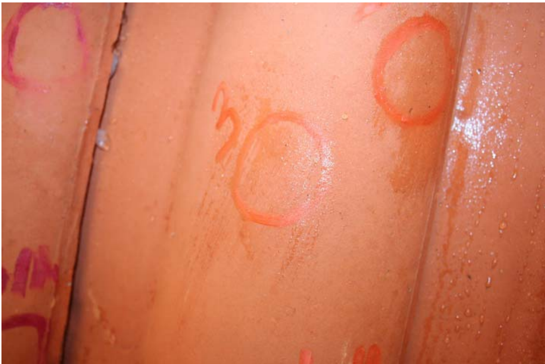
A-40. Tile 3 at impact 3 with 1-3/4 inch ice ball.
